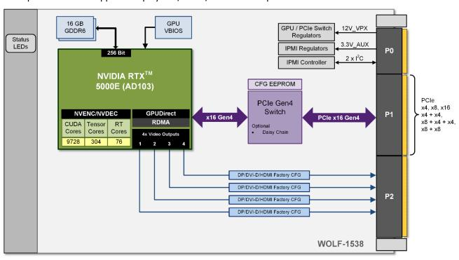
The SOSA Aligned HPC model supports slot profile 14.6.11 with up to PCle Gen4 support.
