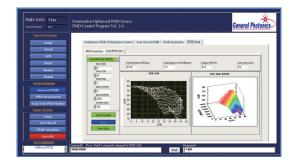
Figure 4. 3D graph display of a DGD/SOPMD scan
