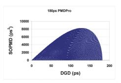
Figure 1. DGD and wavelength independent SOPMD range (180 ps  $PMDPro^{TM}$ )
