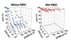
Figure 6. Measured DOP (without PMDC and with PMDC) of a 40-Gbit/s RZ-DQPSK signal versus DGD and SOPMD.
